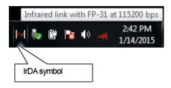
The IrDA symbol changes to an animation icon that shows communication, and when the cursor is pointed over the symbol, the message "Wireless link with FP-31 at xxxx bps" is displayed.
