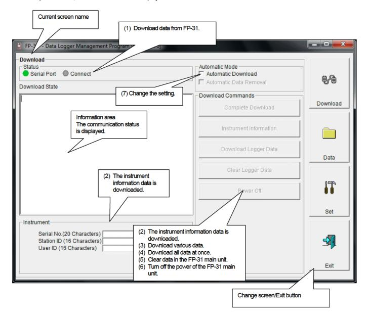
To perform data communication, place the FP-31 main unit to an appropriate position, and with the program activated, turn on the power of the main unit. The program automatically judges whether or not communication is possible. If possible, the PC will be ready to receive the data.
